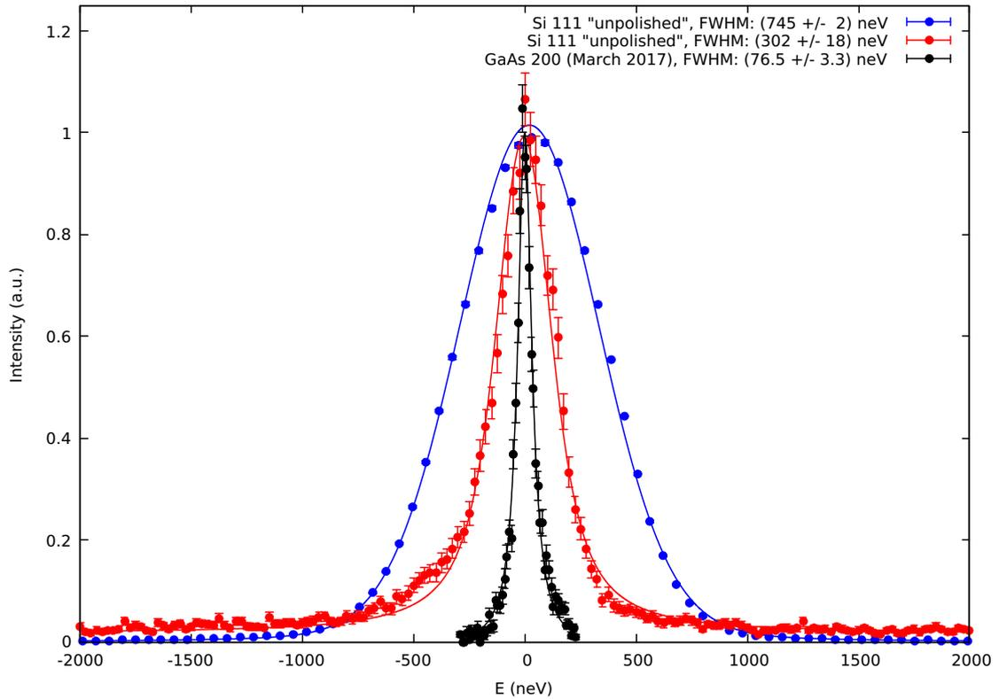
Figure 1: Comparison of the resolution functions of the two standard Si 111 configurations and GaAs 200. Slight asymmetry towards positive energy transfers in GaAs resolution may result from misalignment of the crystals; This will be under further investigation.
