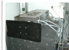
Linear motor Doppler drive by AEROLAS
